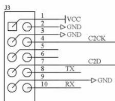
The board firmware can be reprogrammed via J3 using the standard USB programmer available from Silicon Laboratories. On pins 8, 9 and 10, which are not used for programming, a 3.3V level RS232 interface is available.
