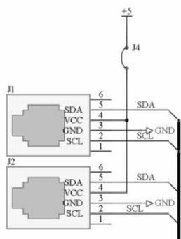
There are two RJ-45 I2C connectors wired in parallel. Having two connectors allows to daisy-chain multiple boards.
