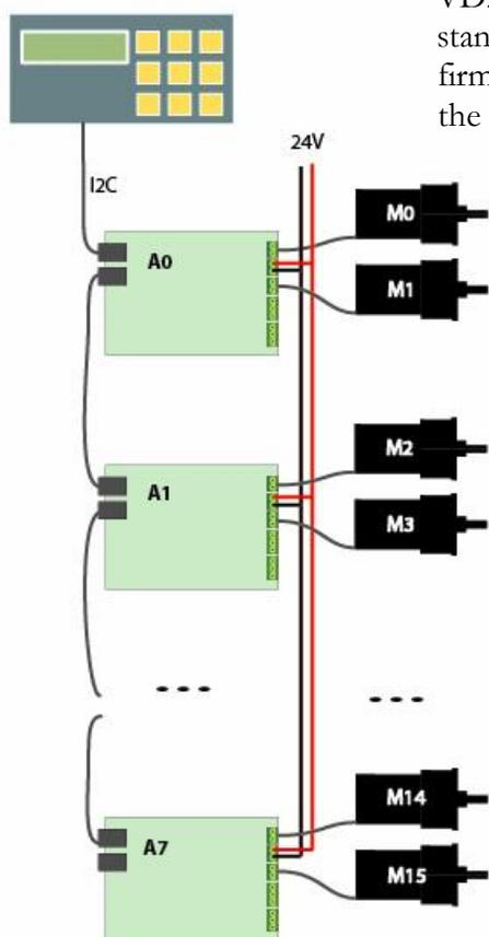
VD203 is used in two basic configurations : master/slave and standalone. Off the shelf, the board is shipped with slave firmware. When assembling master/slave systems, grounding the boards is a critical issue. The problem arises from the motor ground currents affecting the i2c bus. For best results, all boards should be mounted on a metal plate with conductive standoffs, providing low impedance paths for the ground currents.
