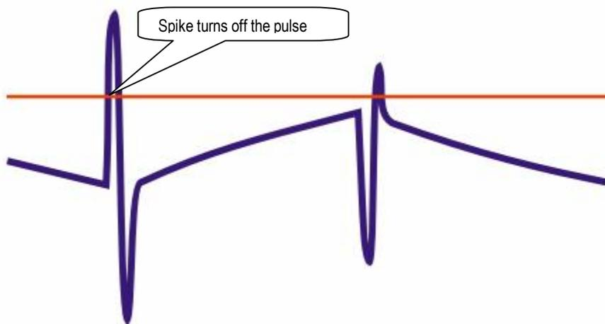
These spikes fool the current limit circuitry into thinking that the limit has been reached and turn off the PWM pulse prematurely. The result is that the PWM stays at minimum duty cycle and the motor barely moves or doesn't move at all.
